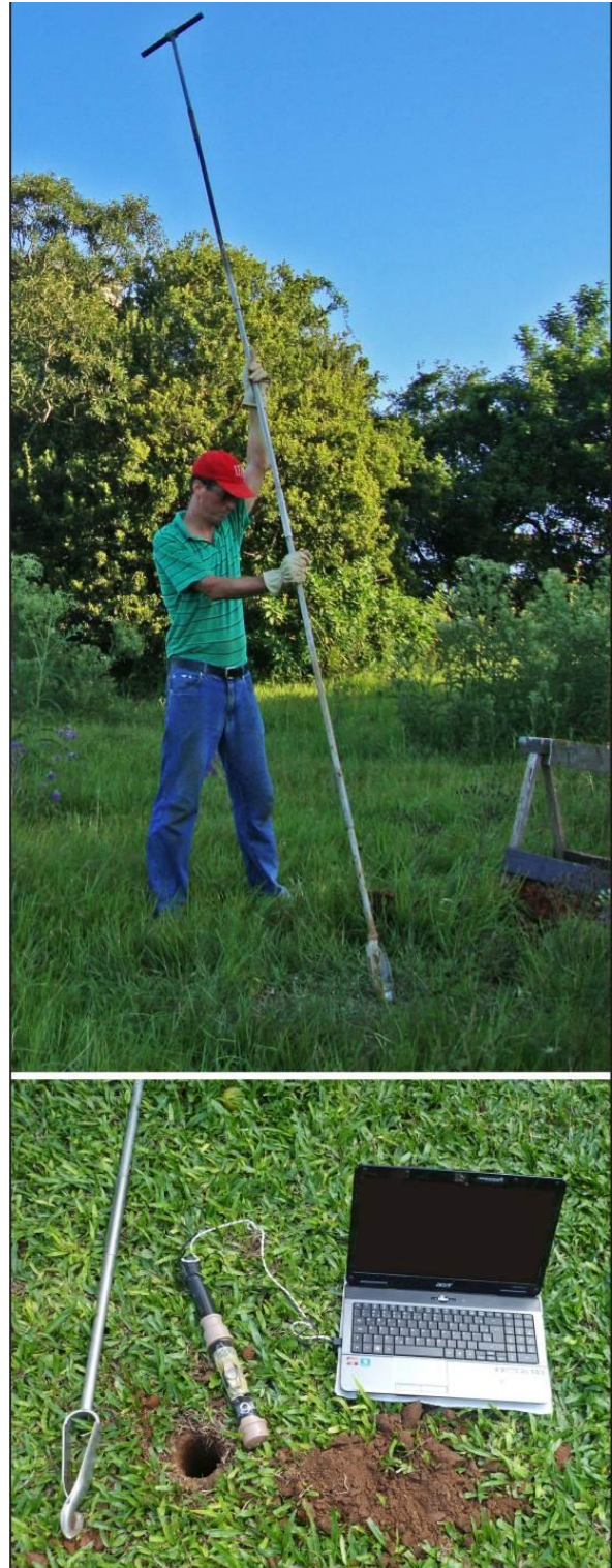
Fig. 6: Investigation of deep tunnels was carried out with boreholes made with an auger. When a tunnel is found, a probe with a headlight and a webcam connected to a laptop is lowered in the borehole to shot pictures.
