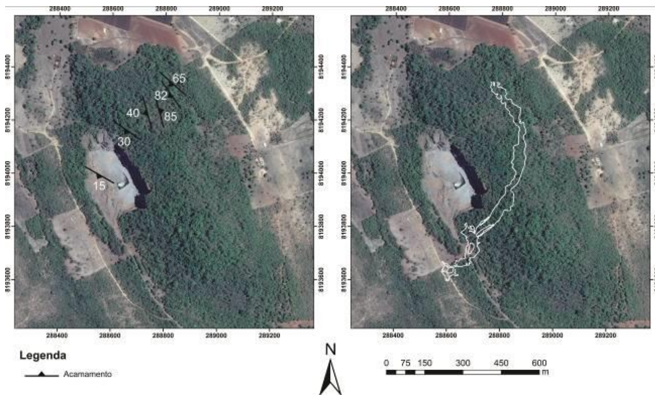
Figure 2: Left: Some attitudes measured on the hill and abandoned mine; Right: Tamboril Cave positioning in relation to the hill.
