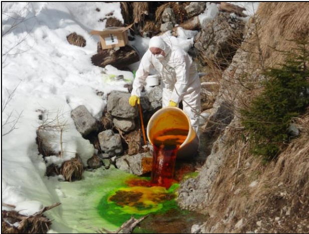
Figure 4: Example of dye tracing of ponor in Slovenia; tracer tests are essential to know the directions of underground water flows.
