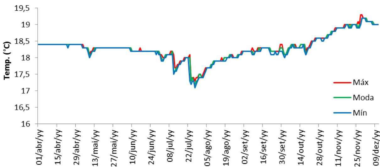
**Figure 9** – Simplified series of water temperature at station in the river gallery, with measures of dispersion (maximum and minimum) and central tendency (mode) for the period from April 1 to December 11, 2009.
