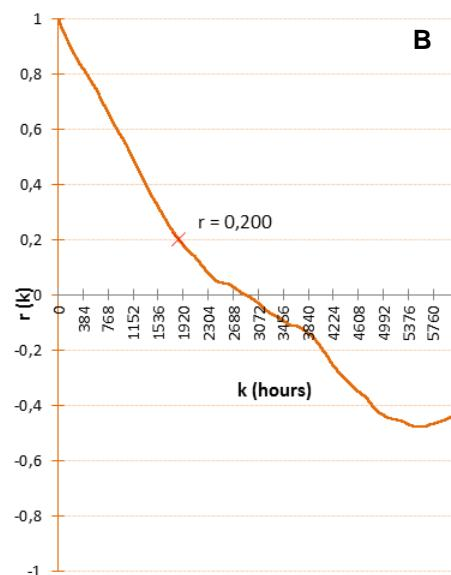
**Figure 10** –original temperature series for the water and the moving average (A) and respective autocorrelation function (B) for the period from April 1 to December 11, 2009.
