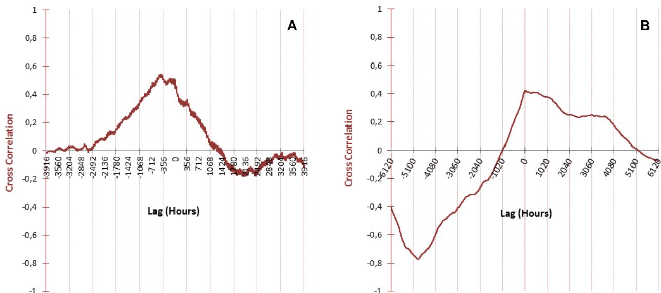
**Figure 11** – Cross correlations between external air temperature and that at the collection point in the gallery of the river (A) and between that of the air in the gallery of the river and that of the water (B)
