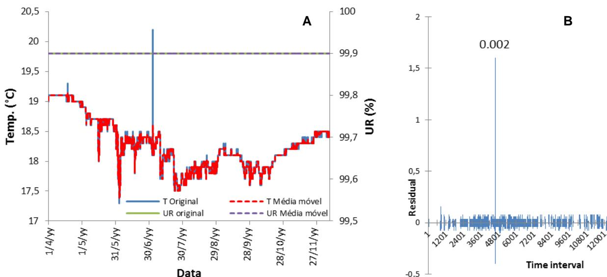
**Figure 7** – Original series for temperature (T) and relative humidity (RH), showing moving averages (A) and the graphs of the respective residuals from smoothing x moving average (B) measured at the station in the gallery of the river for the period from April 1 to December 11, 2009.
