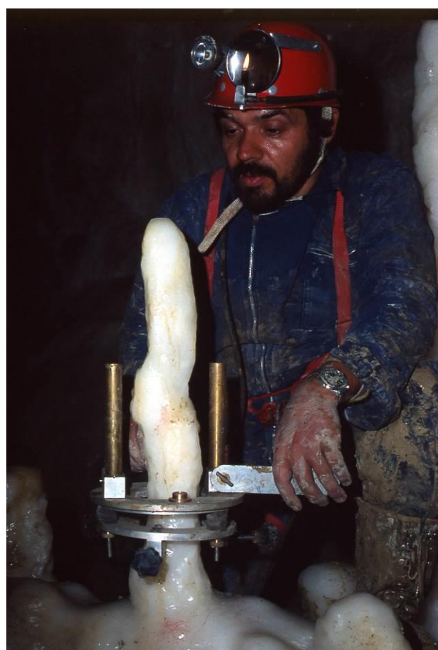
Fig. 16 – Deflection form verticality of the stalagmite axis may record strong earthquakes of the past
